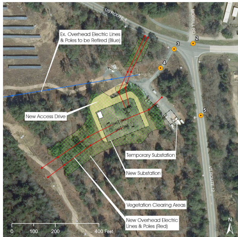
Figure 1: Aerial photo of the new substation site and surrounding area.
