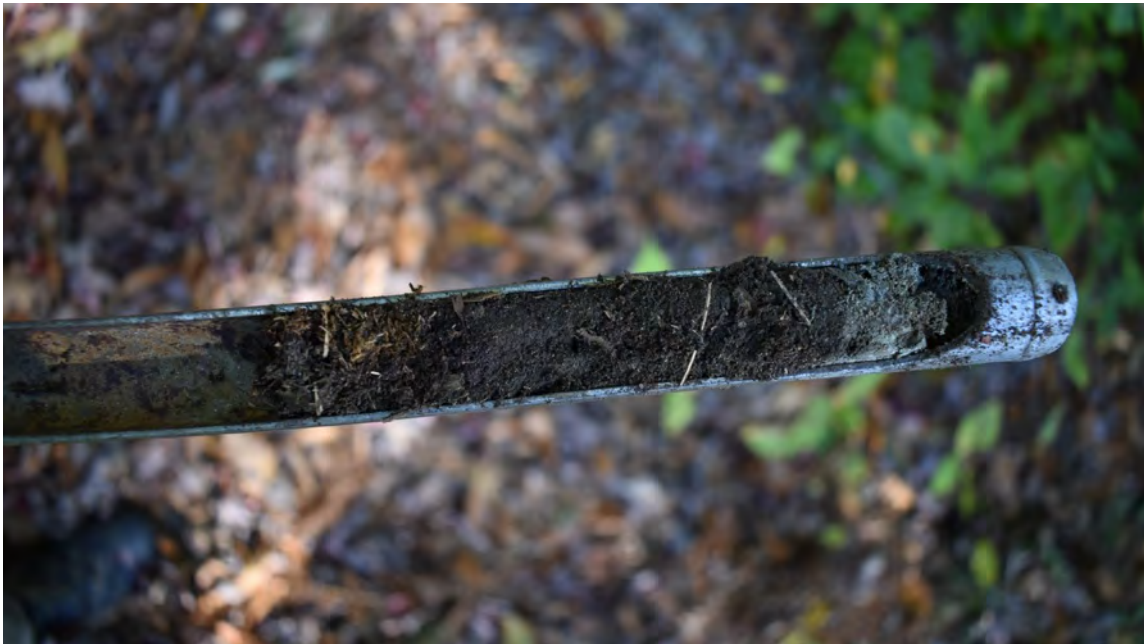
Figure 41. Soil sample taking from just south of the temporary GMP Taftsville substation within the South Study Area of the GMP Taftsville Substation Relocation Project, Woodstock and Hartland, Windsor County, Vermont. Note the gravelly sand just below the 'Ao' horizon.
