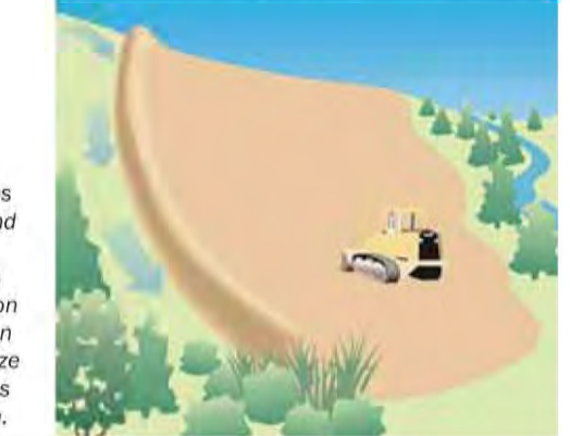
Berms and ditches divert clean upland runoff around construction sites and reduce erosion and sedimentation problems. Stabilize berms and ditches after construction. 15
