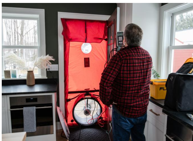
A VGS Building Analyst assessing home airtightness with a blower door test during an energy audit.
