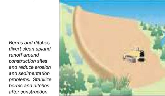
Berms and ditches divert clean upland runoff around construction sites and reduce erosion and sedimentation problems. Stabilize berms and ditches after construction. 15
