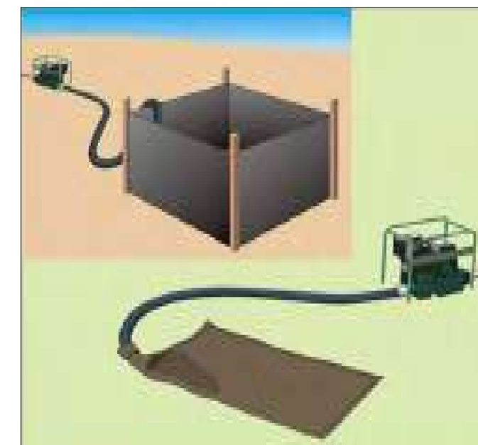
Water is pumped from the construction site into a silt fence enclosure on a vegetated area or into a sock filter away from waterways.
