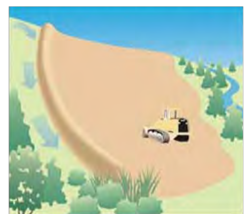
Berms and ditches divert clean upland runoff around construction sites and reduce erosion and sedimentation problems. Stabilize berms and ditches after construction. 15
