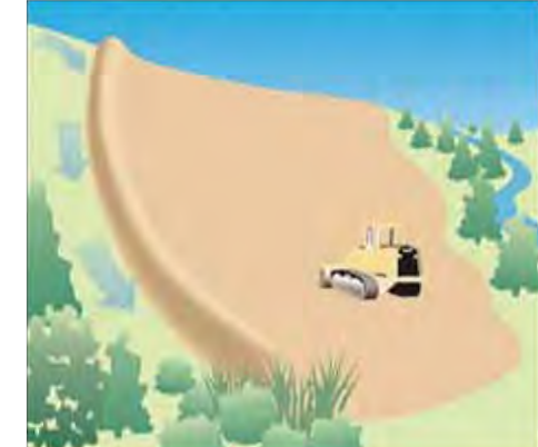
Berms and ditches divert clean upland runoff around construction sites and reduce erosion and sedimentation problems. Stabilize berms and ditches after construction.
