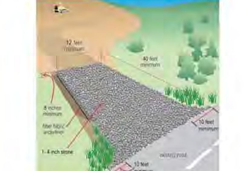
Construction entrance detail. Entrance/exit pad must keep mud from tracking onto both paved and dirt roads.
