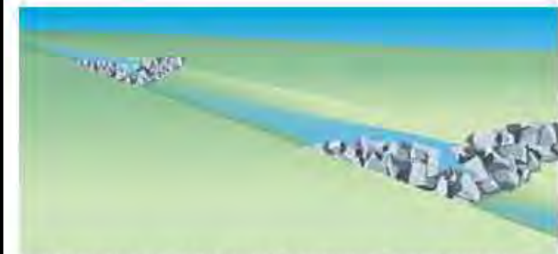
Rock check dams must be installed before excavation or fill activities begin. See "How to install" for spacing directions.
