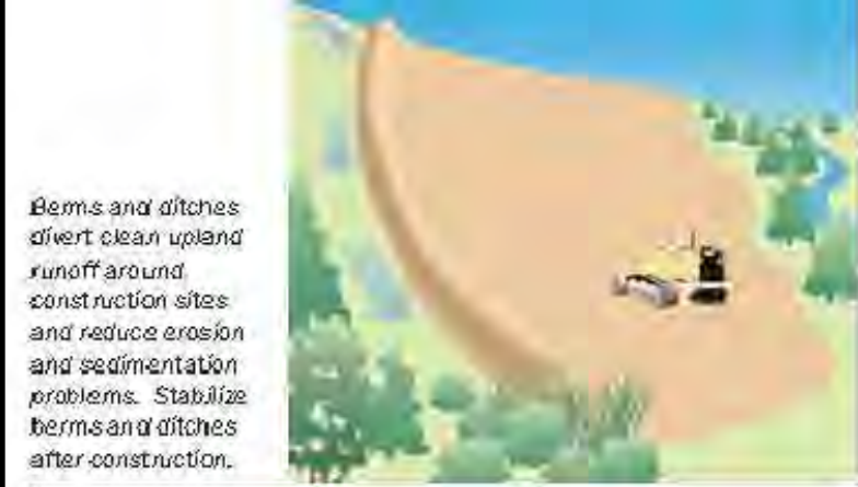
Berms and ditches divert clean upland runoff around construction sites and reduce erosion and sedimentation problems. Stabilize berms and ditches after construction.
