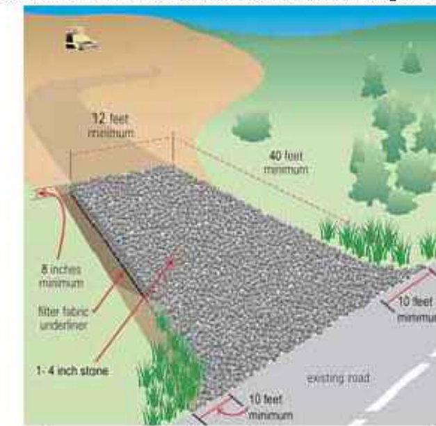
Construction entrance detail. Entrance/exit pad must keep mud from tracking onto both paved and dirt roads.
