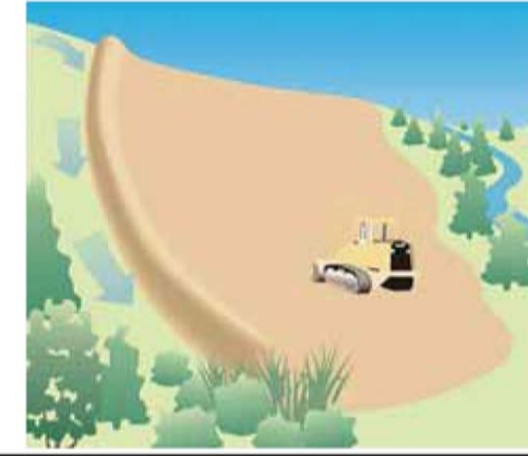
Berms and ditches divert clean upland runoff around construction sites and reduce erosion and sedimentation problems. Stabilize berms and ditches after construction.
