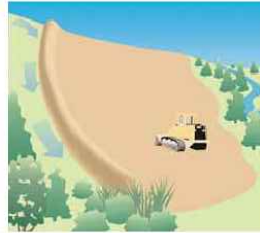
Berms and ditches divert clean runoff around construction sites and reduce erosion and sedimentation problems. Stabilize berms and ditches after construction.
