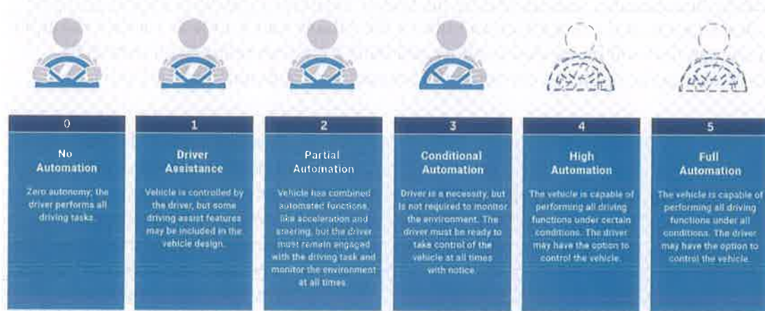
Figure 2.6 Vehicle Automation Levels. Levels 1 and 2 are already common on the roadways of Vermont.
