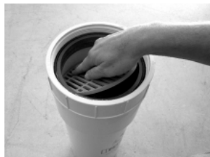
The pre-filter material is below the grate. Remove the grate by pushing down on one side and lifting straight up.
