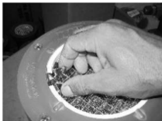
Remove the retaining ring by squeezing the metal tabs together and lift.
