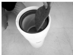
Replace with new materials. The gray Adsorb-It® disk goes on the bottom, followed by loose filter floss. Next place the 4in. thick floss disk, then the black Flo-Free Mesh. Replace the grate.
