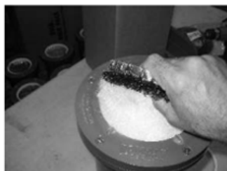
Remove the grate, the soiled mesh and floss.
