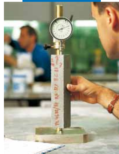
Determination of retained expansion according to UNI 8147
